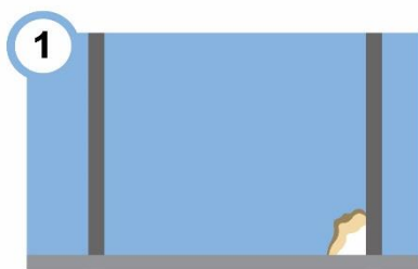
1 Damage to corner of Shaft Liner panel
