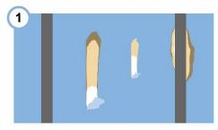
Ripped, torn or scrapped Shaft Liner panel face paper
