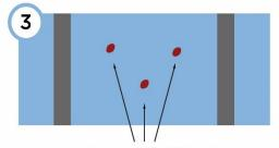
Patch nail holes with 3M Fire Barrier Sealant CP 25WB+ fire caulk
