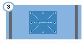
Center minimum 12" x 12" piece of 1/2" M-Bloc Ekcel Type X wallboard over the filled hole and secure with 1 ½" Type G laminating screws spaced 6" o/c
