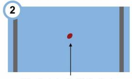
Fill entire hole with 3M Fire Barrier Sealant CP 25WB+ fire caulk
