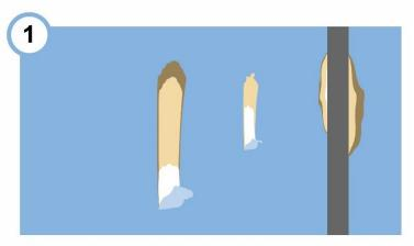
No repairs needed to ripped, torn, scrapped or missing paper on the 1/2" M-Bloc Ekcel Type X wallboard panels
