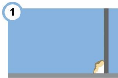
1 Damage to corner of 1/2" M-Bloc Ekcel Type X wallboard
